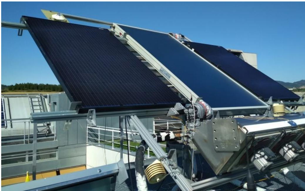
Figure 7 Assembly of solar components at fixed tilt. Left, PV module. Center, Solar Thermal collector. Right PVT collector. Testing location: Sarriguren, Spain Latitude 42,8^{\circ} Longitude -1,6^{\circ} .
