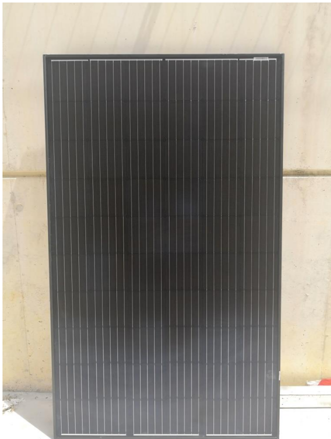
Figure 1. PVT sample. PVT collector composed by PV module Canadian Solar CS6K-295MS, serial number: 11810481170589 and Heat exchanger P-FHE16PS, serial number: 100122190621.
