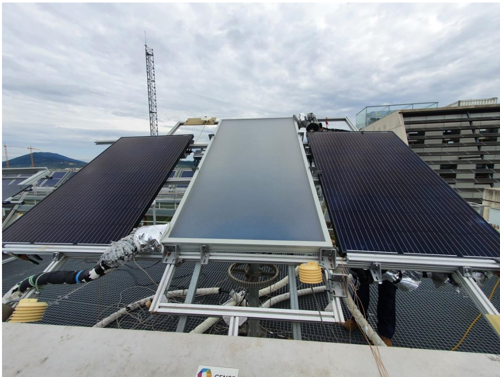
Figure 3. Assembly of solar components at fixed tilt Testing location: Sarriguren, Spain Latitude 42,8° Longitude -1,6°
