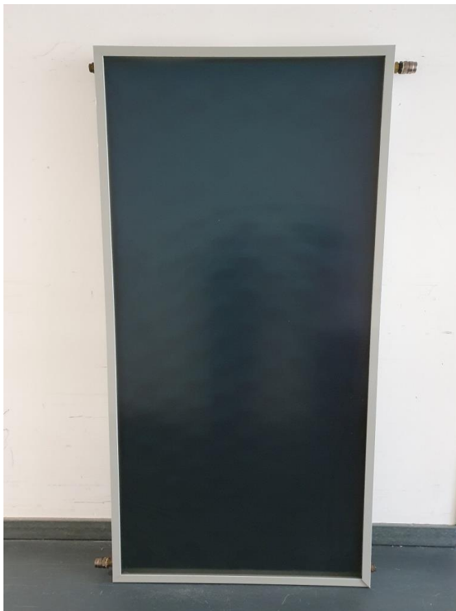
Figure 2. Solar Thermal Collector, Sammler Aris 2004 serial number: 103.739
